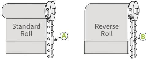
If your blind features a child safety chain connector instead of an endless loop, make sure it is positioned correctly *before* putting the control end back into the tube. For standard roll fabric, it needs to be positioned at the back of the loop (A). For reverse roll fabric, it needs to be positioned at the front of the loop (B). To do this, hold the control end and pull the chain round to the correct position as illustrated. See step 5 for a further explanation of standard and reverse roll.
