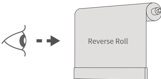
'Reverse' roll is where the fabric rolls down off the front of the tube thereby hiding the roll of fabric. This method gives added clearance at the back of the blind for obstructions such as window handles. This is particularly useful when the blind is fitted inside of the window recess.
