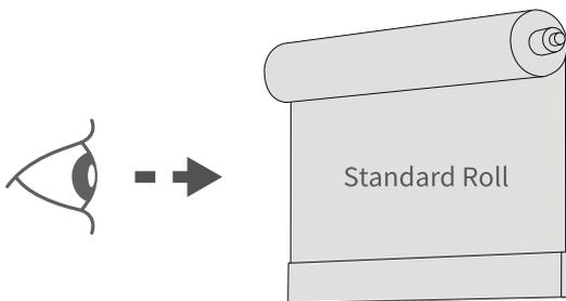
The fabric of our roller blinds can be rolled onto the tube in two different directions. 'Standard' Roll is where the fabric rolls down off the back of the tube so that it's closest to the window or the wall. This is particularly useful when the blind is mounted outside of the window recess as there will be less light leakage.
