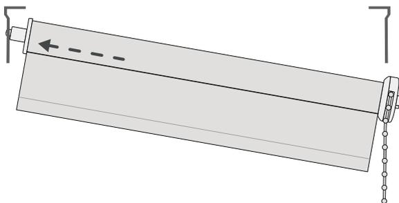
Holding the blind, locate the pin end into the central round hole of the corresponding bracket and push it in all the way.
