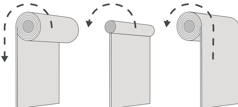
To change the direction of the roll, simply pull on the chain until the fabric is rolled all the way down fully exposing the aluminium tube. Once all the way down, hold the bottom of the fabric by the bottom bar to keep it taut and then proceed to keep on rolling in the same direction until the fabric has rolled all the way up the other side of the tube. Note that doing this will now reverse the direction you will need to pull the control chain for lowering and raising the blind.
