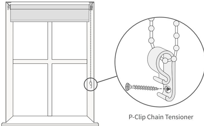
The P-Clip chain tensioner must be fitted at the maximum distance possible from the control mechanism to prevent the chain loop from becoming slack.
