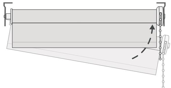
With the pin end now in position, lift the control end and insert it into the opposite bracket ensuring the lugs click into their corresponding slots. Make sure the centre lug is in the vertical position.
